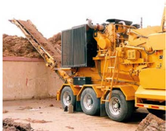
Figure 82. The trunk pieces are shredded into very small bits and dumped in a square
